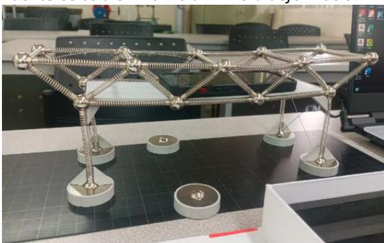
Ríos, K., Carrera, H., Beltrán, L., & Lara, E. (2025). COMPARATIVE ANALYSIS OF THE DEFORMATIONS OF A TRUSS BRIDGE USING THE MOLA KIT AND SAP 2000.
